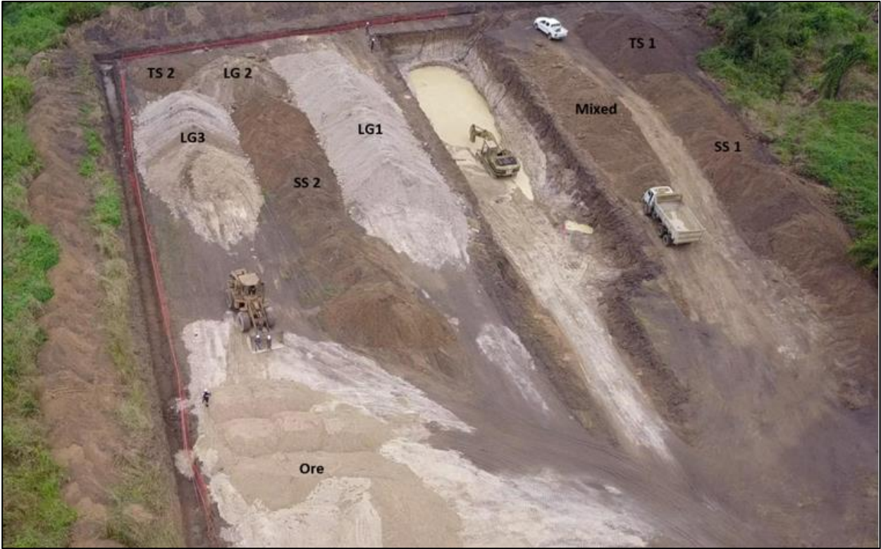
Figure 2 – Cácata mine site and pit design with works being undertaken for the 250-tonne bulk sample.
