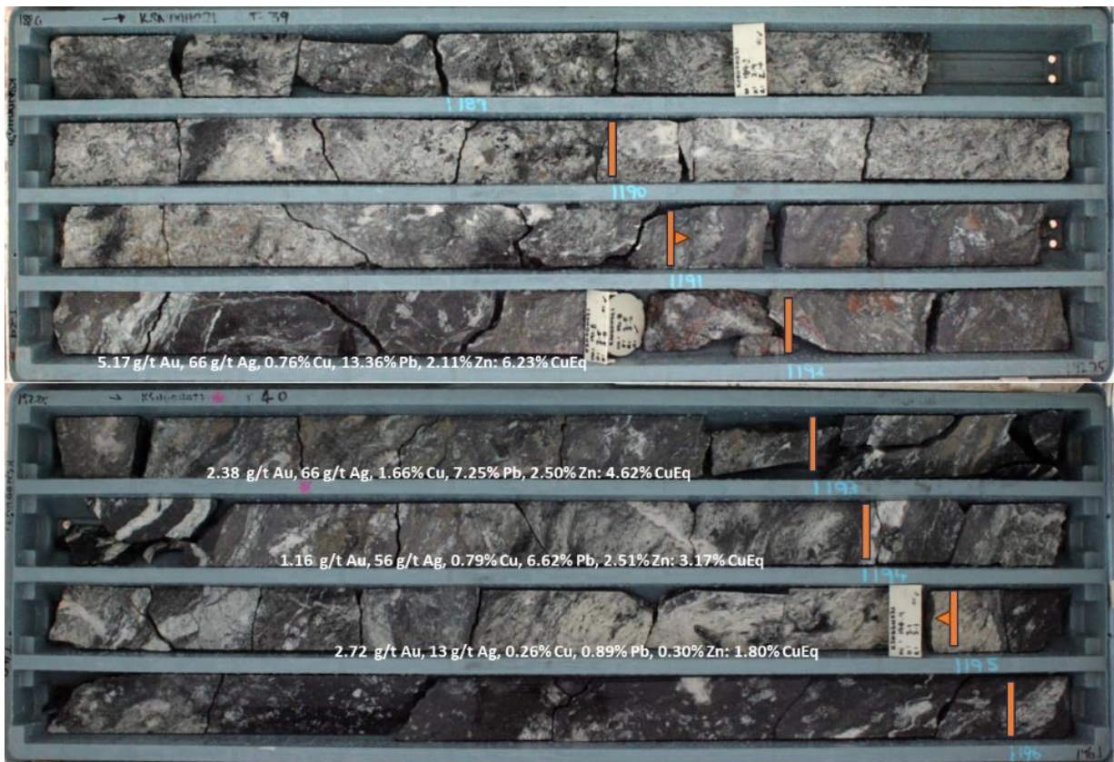
Figure 7: Drill core from KSNDDH021 (4m wide sulphide rich breccia lode (estimated true width of 2m) within a broader 31.6m wide brecciated and veined lode zone from 175.3mdh).
