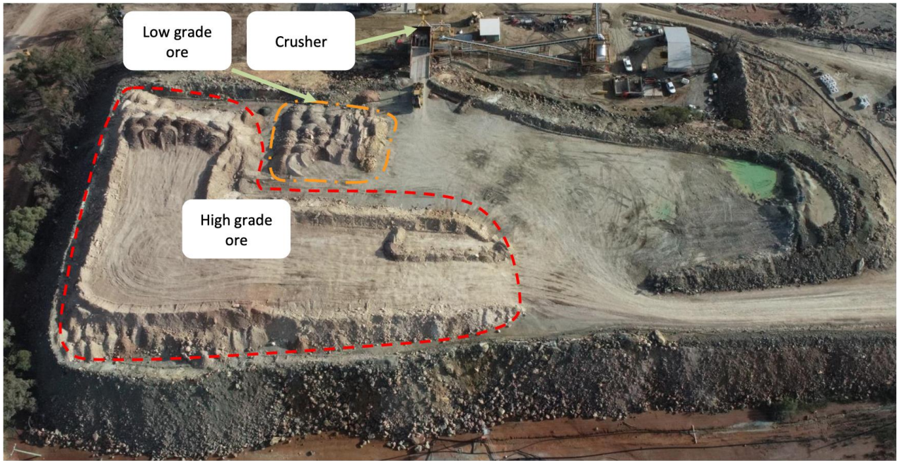
Figure 3: Stockpiled oxide ore on the ROM pad.
