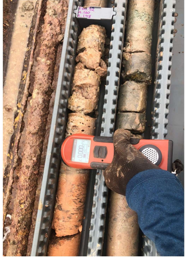
Figure 2: Magnetic susceptibility test on drill cores.
