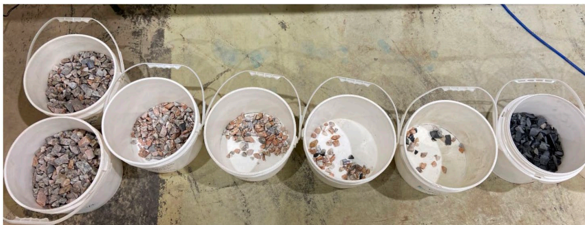
Figure 5 - Dynamic XRT ore sorting results showing separation of pegmatites (left) from waste rock (right).
