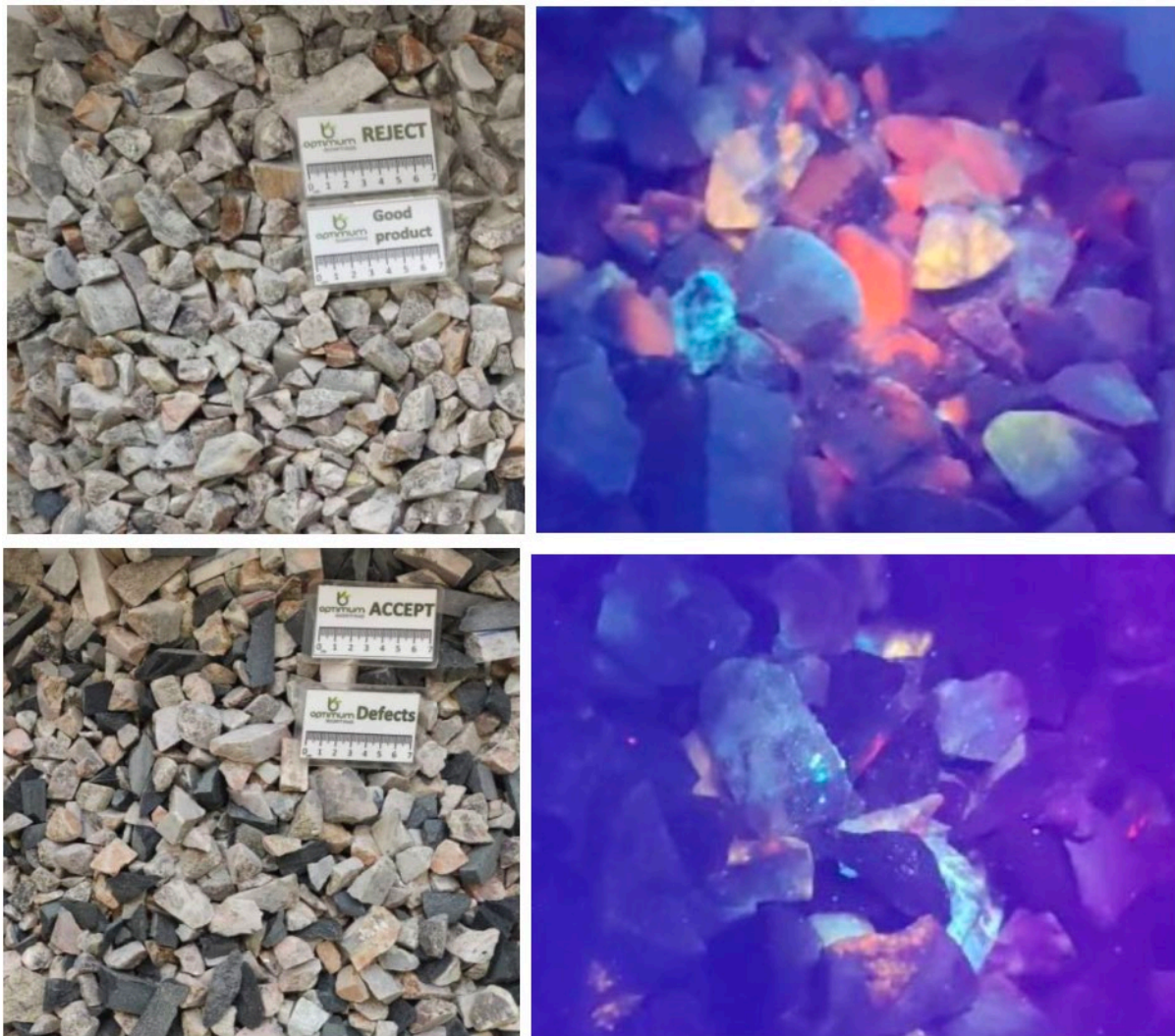
Figure 6 - Dynamic UV ore sorting trial results showing spodumene ore concentrate with its characteristic UV response (top) and waste minerals with no response (bottom).
