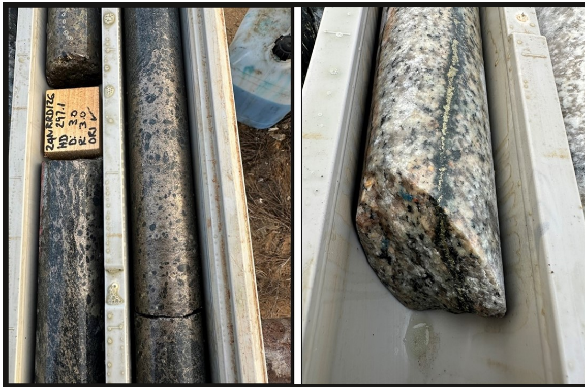
Figure 1 – Massive (left) and veined (right) sulphide mineralisation within hole 24NRDD0126 contained within interval 295.1 -300.3m (5.2m).
