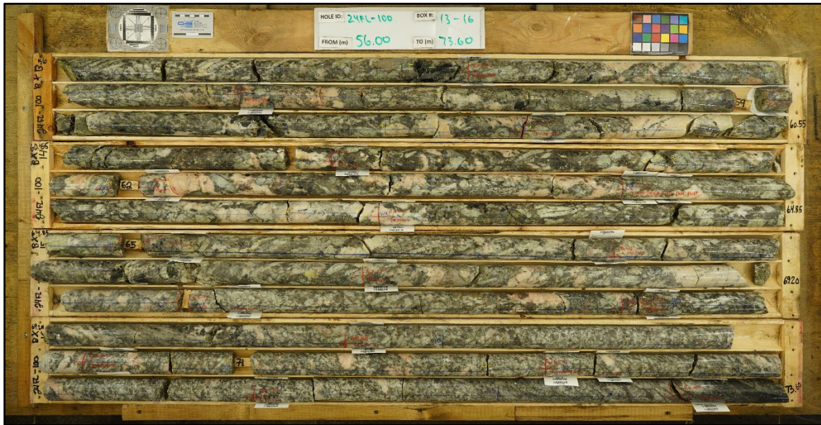
Figure 4 – Core box containing spodumene grading 1.88% Li 2 O in hole 24FL-100, Falcon Little Lake (refer to Appendix 1, Table 1, significant intercept table).
