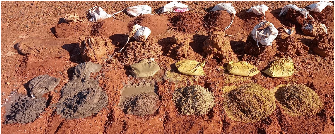
Figure 6: 24YRAC048 Detail of redox boundary over 60-66m interval showing reduced carbonaceous clays (LHS) grading downwards into strongly oxidised gravelly sands (RHS). Mineralisation occurring above reduced carbonaceous sediments is interpreted as equivalent to Maningee’s ‘A Roll’ with the clay horizon serving as an aquiclude that compartmentalises the palaeochannel aquifer.
