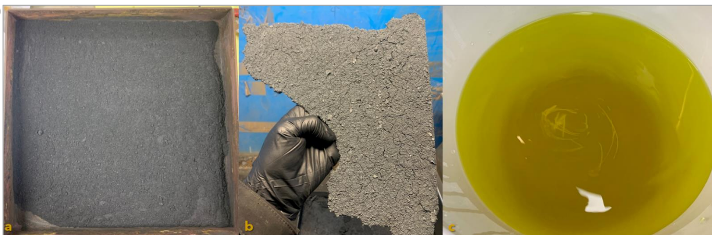
Figure 1; Photos showing a) Magnetite Concentrate prior to roasting, b) calcine product post roasting, and c) Vanadium bearing solution after leaching.
