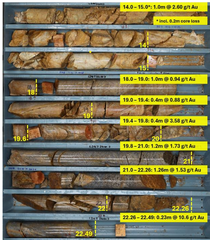
Figure 4 - LZGT24003 Tray 6 (upper 3 rows) and Trays 8-10 (lower 7 rows) displaying typical Link Zone oxide/transitional mineralised zones within broader 8.49m @ 1.56g/t (from 14m) intercept at Merriyulah
