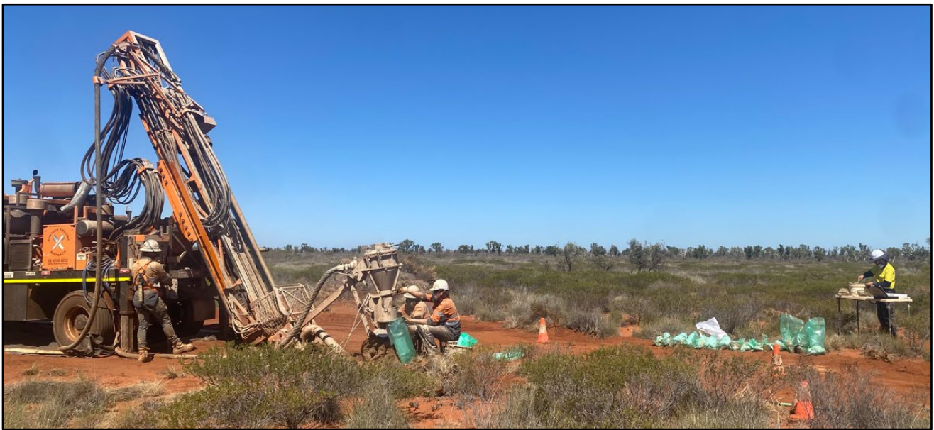
Figure 1: Air Core rig completing the last exploration hole of Phase 1 at NAE's Wagyu Gold Project
