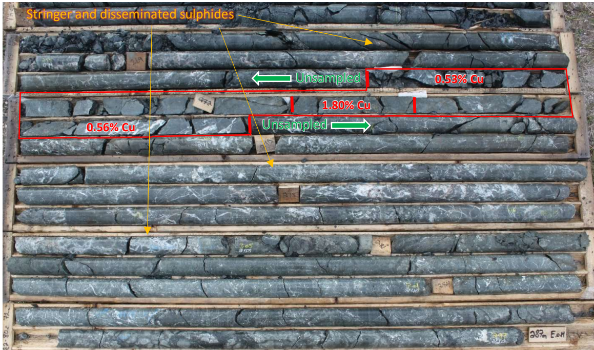
Figure 4: Previous Drill Hole YH22 - 080 showing extent of unsampled intervals with sulphides adjacent to ore zone 1 (Cont)
