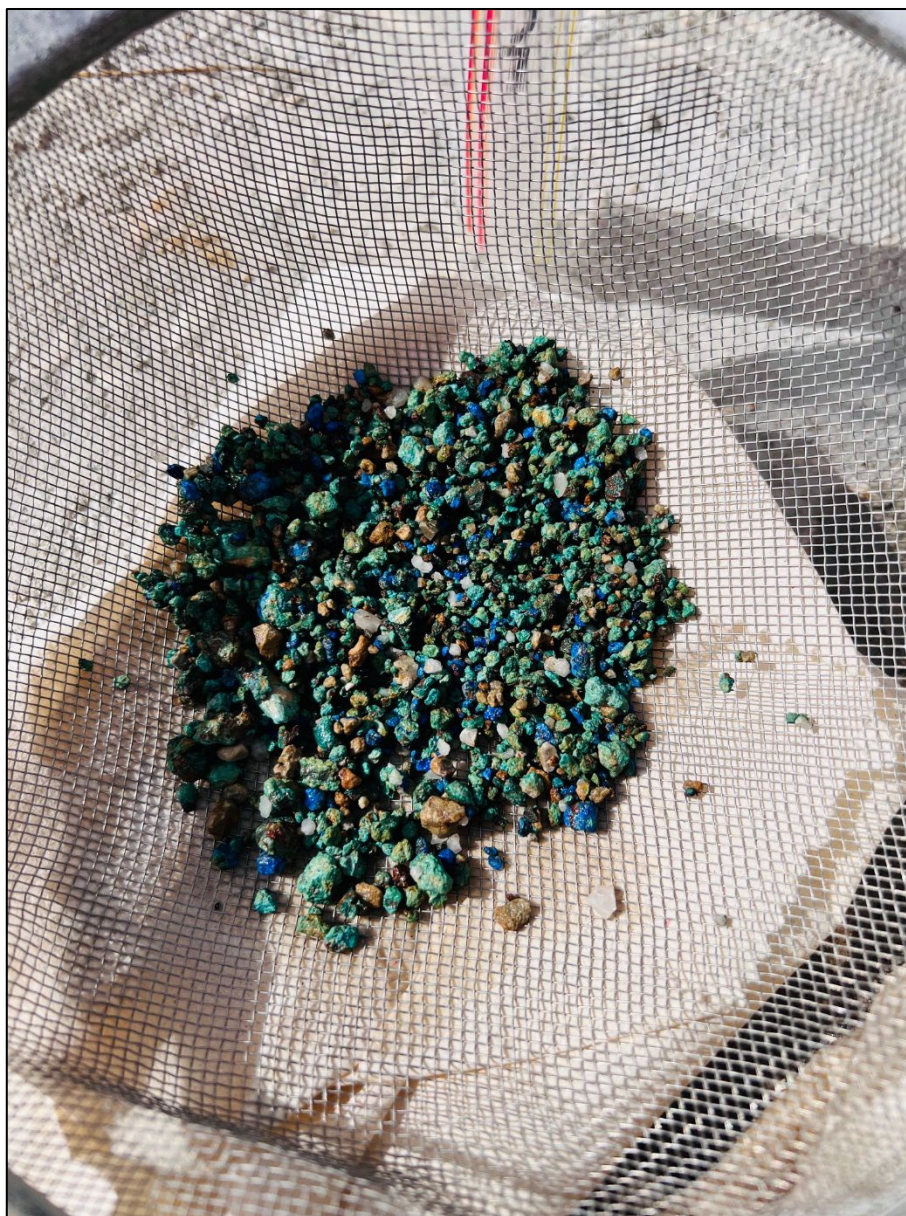
Photo 2. Close up of SJAC112 16-17m showing distinctive azurite and malachite copper oxide minerals. Note that the sieving washes away the clay component of the sample and that the percentage of material remaining in the sieved component is upgraded as a proportion of the total sample. Sieve is approximately 150mm in diameter.
