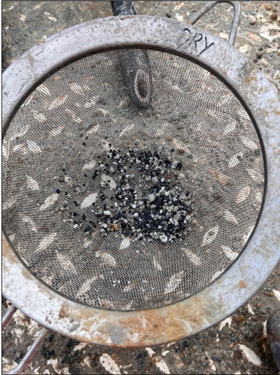
Photo 3. Sieved material from SJAC117 41-42m showing +50% covellite-coated (dark blue / black) chalcopyrite (yellow) grains. Note that the sieving washes away the clay component of the sample and that the percentage of material remaining in the sieved component is upgraded as a proportion of the total sample and therefore likely over-represents the sulphide content. Sieve is approximately 150mm in diameter.
