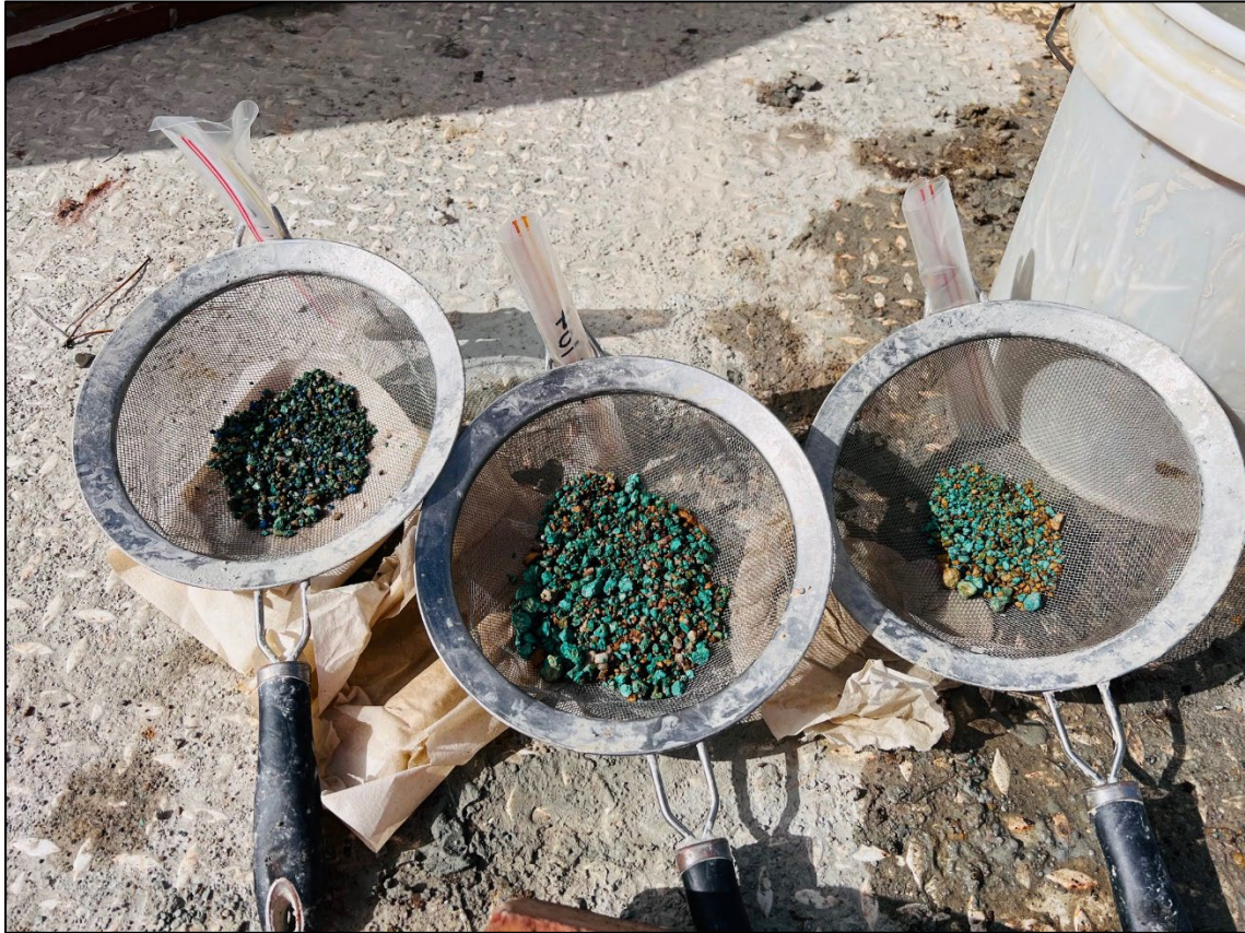
Photo 1. Sieved aircore chips from (L-R) SJAC112 16-17m with azurite (blue) and malachite (green), SJAC104 2-4m, and SJAC103 19-20m. Note that the sieving washes away the clay component of the sample and that the percentage of material remaining in the sieved component is upgraded as a proportion of the total sample. Sieves are approximately 150mm in diameter.
