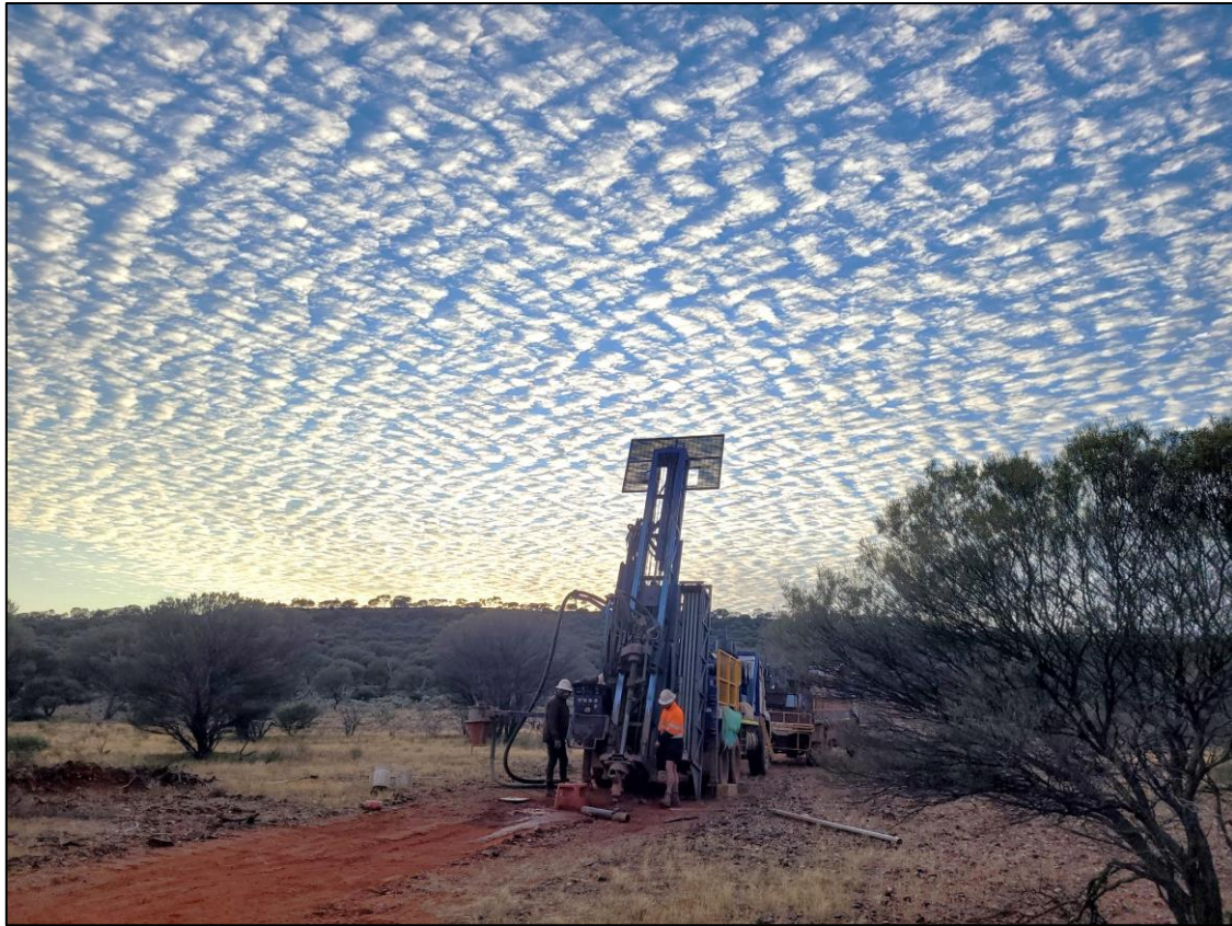
Figure 2: Reconnaissance aircore drilling during August in typical shallow colluvial terrain at Box Soak.
