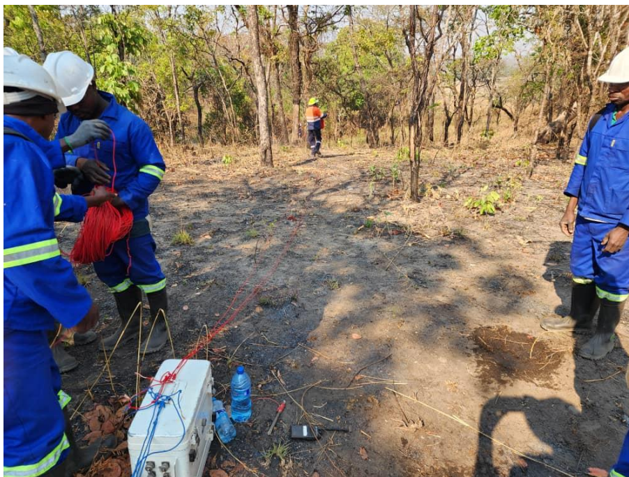
Figure 5: IP surveying underway at the Kapikuba Prospect
