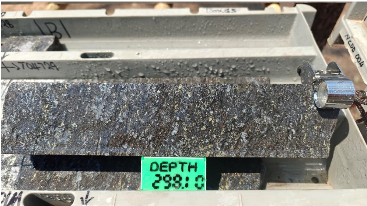
Figure 1. High grade copper mineralisation (as chalcopyrite) in Ore Schist unit from Nyungu Central (Hole NCDD004; core shown from downhole depth 298.1 metres)
