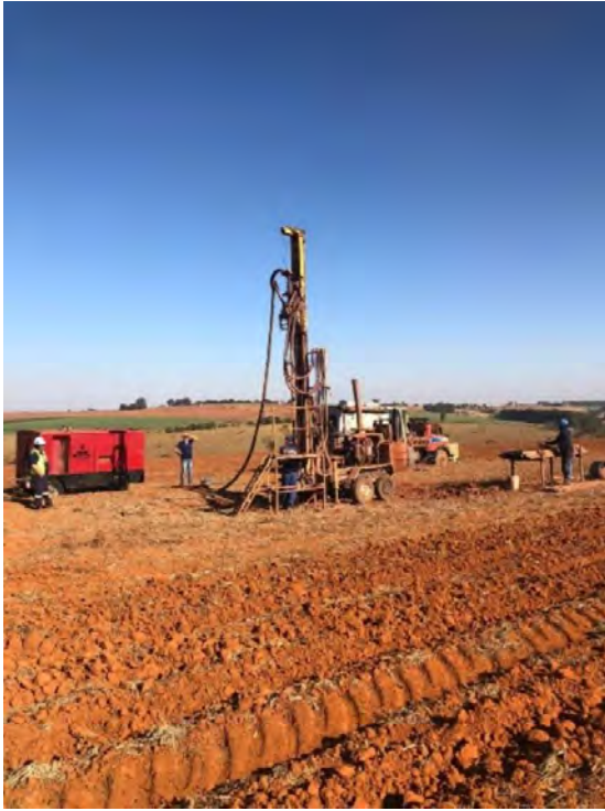
Figure 6: RC drilling in operation in CODA North
