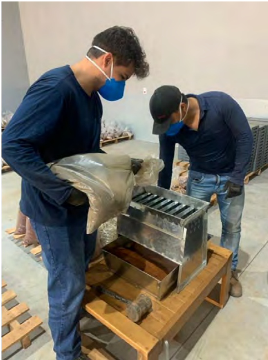
Figure 8: Enova's professional geology team using dry riffle splitter for sub-sampling
