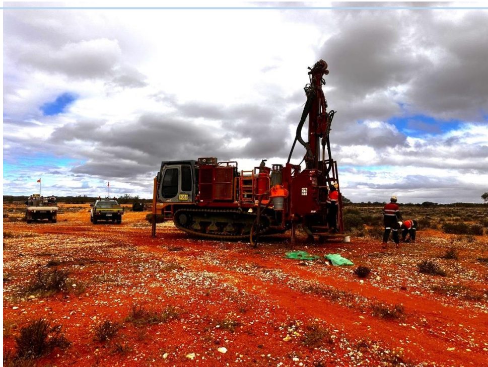
Figure 1: AC drill rig commencing exploration drilling adjacent to North Stanmore on 5 th September 2024
