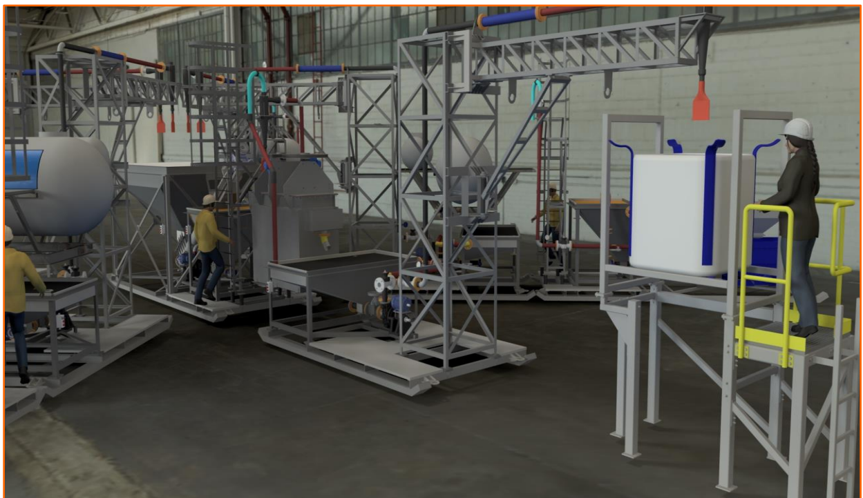
Figure 3: Conceptual 1 TPD Flash Joule Heating Pilot Facility – Inside the Plant
