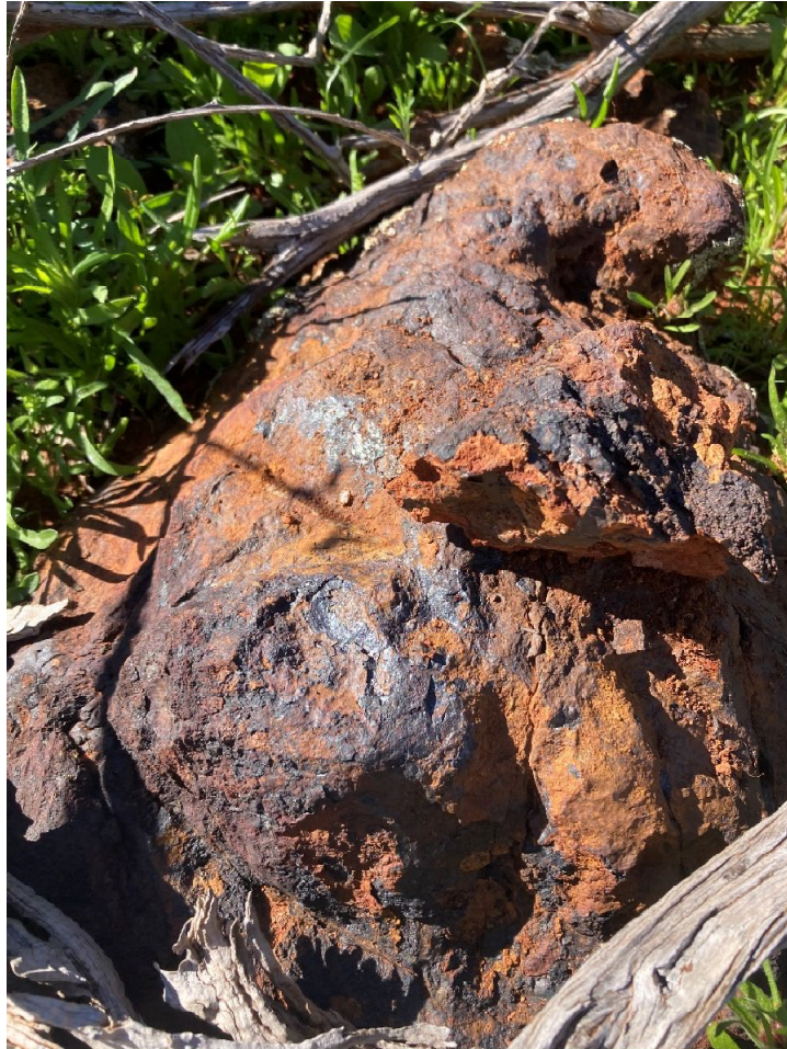
Slide 1: Gossanous sample PBG002: XRF assays of 270ppm Ni, 460ppm Cu, 200ppm Zn (Location 531747E 6752840N)
