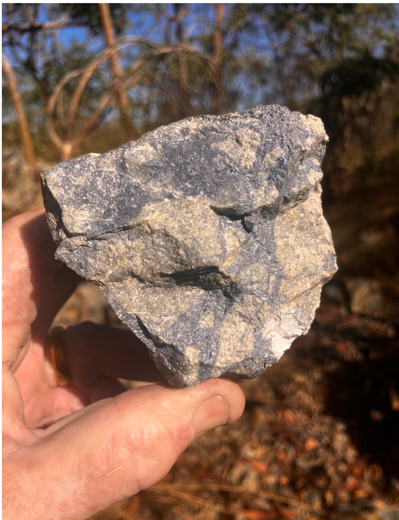
Chloritic altered rhyolite breccia with massive stibnite as matrix infill on southern lode.
