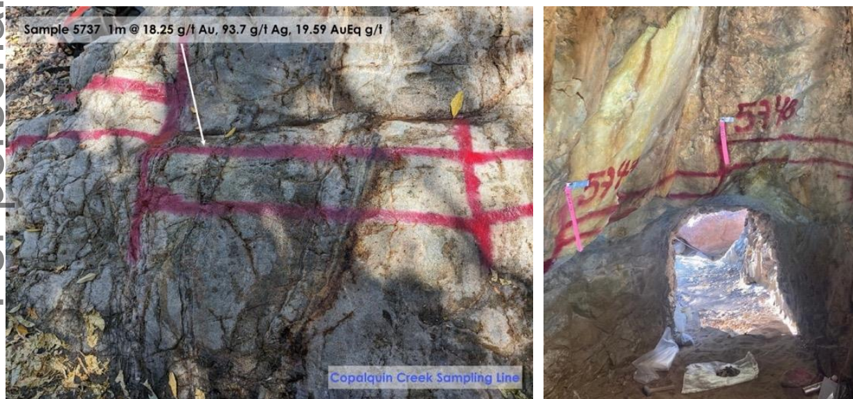
Figure 9 Left: Mineralised structure in the Copalquin Creek important for the overall district geologic model. Right: Inside the historic Copalquin mine showing diamond saw channel sample.
