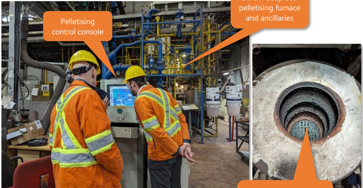
Figure 2: Corem pelletising pot grate furnace and control console
