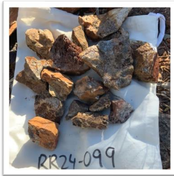
Figure 3. Rock chip RR24-099, taken for gold mineralisation at the Sabre Gold Prospect. Sample contains 3.3g/t Au.
