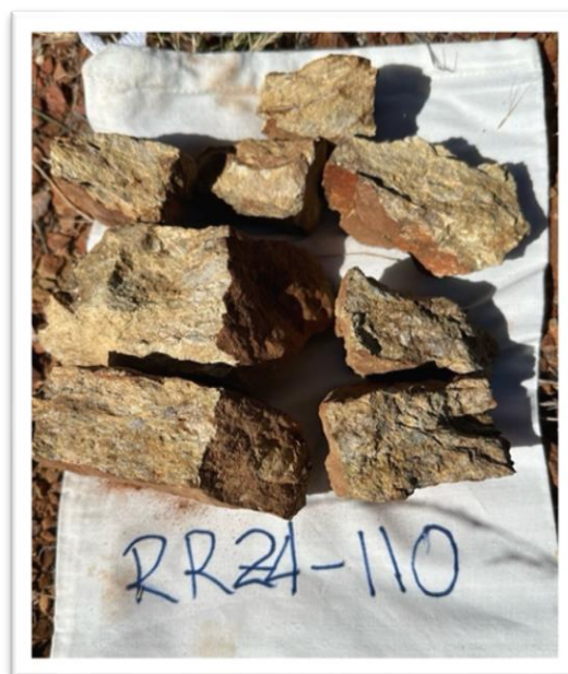
Figure 4. Rock chip RR24-110 taken for gold mineralisation at the Falchion Gold Prospect. Sample contains 12.6% Sb, 1.1g/t Au and 4.0% Pb.
