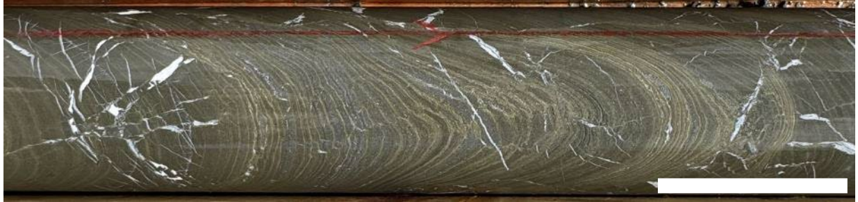
Figure 6: CD24-002 at 118.6m; laminated massive sulphides. The dark green sulphides are predominantly pyrite, the yellow green to brassy-yellow sulphide is chalcopyrite, with white carbonate veins (assayed 5.1% Cu + 12.4 g/t Ag). Scale bar approx. 5cm
