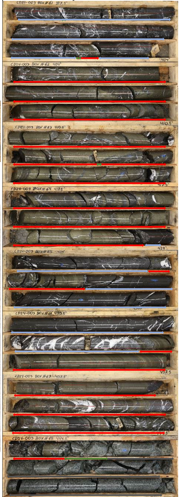
Figure 4. Massive sulphide mineralised intercepts in all core boxes from holes CD24-001, CD24-002 and CD24-003.
