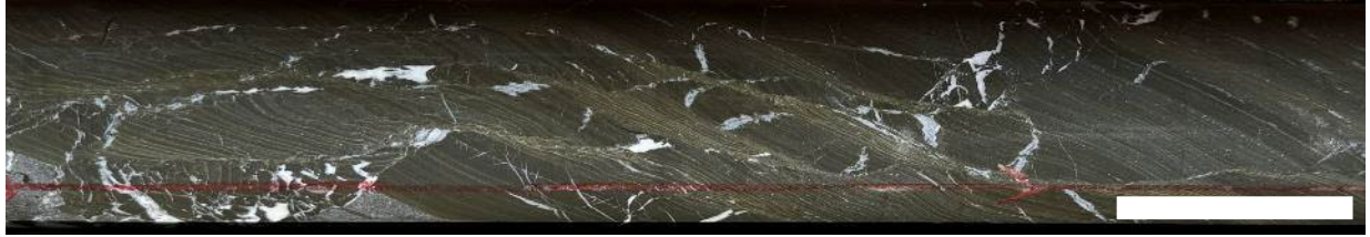
Figure 5: CD24-002 at 118.5m; laminated massive sulphides. The dark green sulphides are predominantly pyrite, the yellow green to brassy-yellow sulphide is chalcopyrite, with white carbonate veins (assayed 6.6% Cu + 15g/t Ag). Scale bar approx. 5cm
