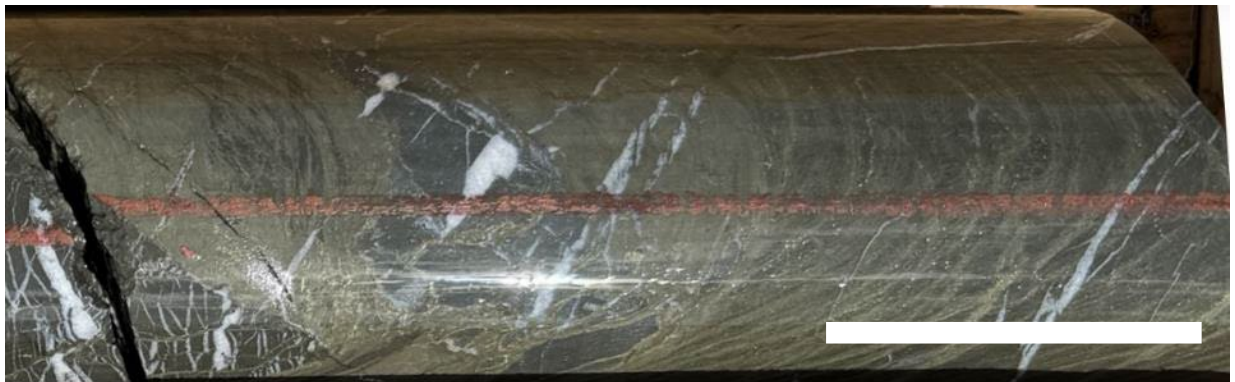
Figure 8, CD24-003 at 124.4m; laminated massive sulphides. The dark green sulphides are predominantly pyrite, the yellow green to brassy-yellow sulphide is chalcopyrite, with white carbonate veins (assayed 15.3%Cu + 29.5g/t Ag). Scale bar approx. 5cm
