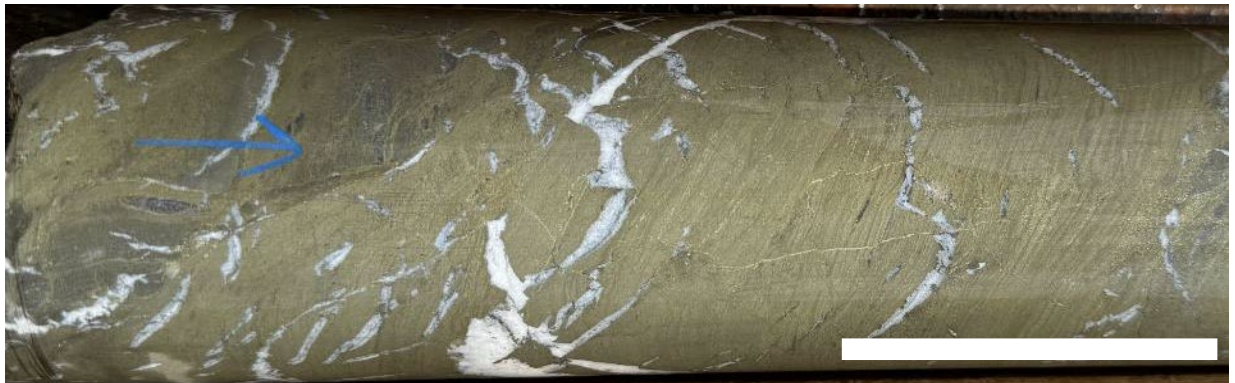
Figure 7: CD24-002 at 119.8m; laminated massive sulphides, predominant brassy chalcopyrite thinly interbedded with pyrite with white carbonate veins (assayed 13%Cu + 21.1 g/t Ag). Scale bar approx. 5cm
