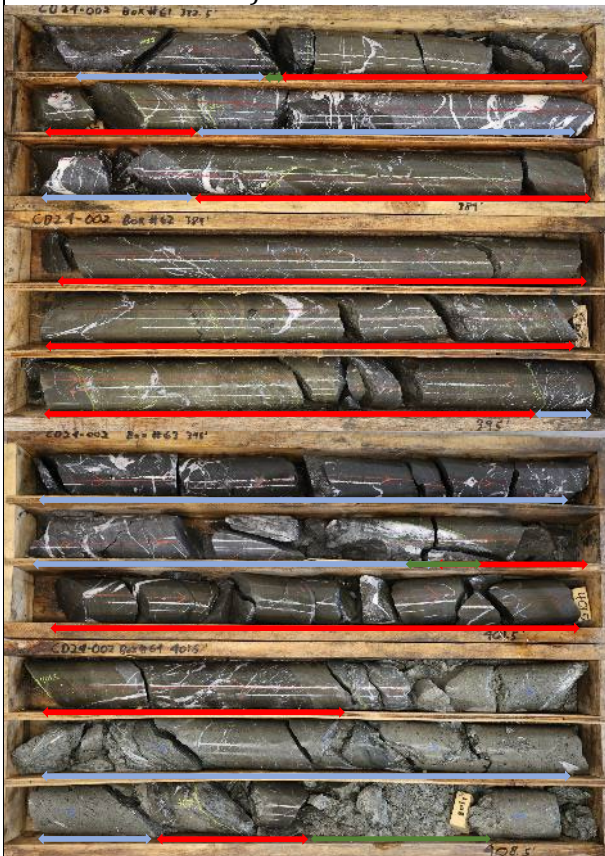
Figure 4. Massive sulphide mineralised intercepts in all core boxes from holes CD24-001, CD24-002 and CD24-003.
