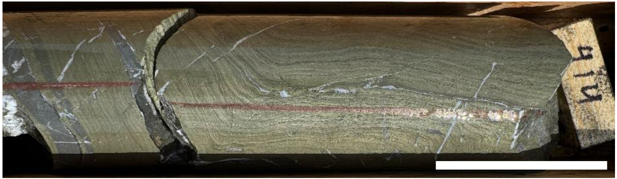
Figure 9: CD24-003 at 126.0m; laminated massive sulphides, predominant brassy chalcopyrite thinly interbedded with pyrite and shale with white carbonate veins (assayed 15.5%Cu + 22.6g/t Ag). Scale bar approx. 5cm
