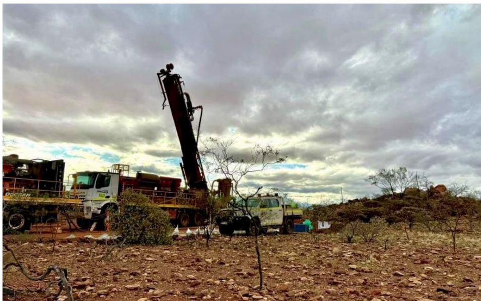
Figure 1: Photo of the Topdrill RC rig drilling at Tiger.
