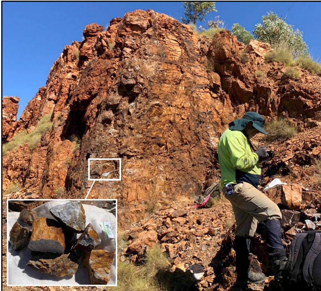
Figure 4 - Sample location 24PS_RS019 (0.41g/t Au) illustrating quartz vein arrays with iron oxide minerals after sulphides in siltstone host
