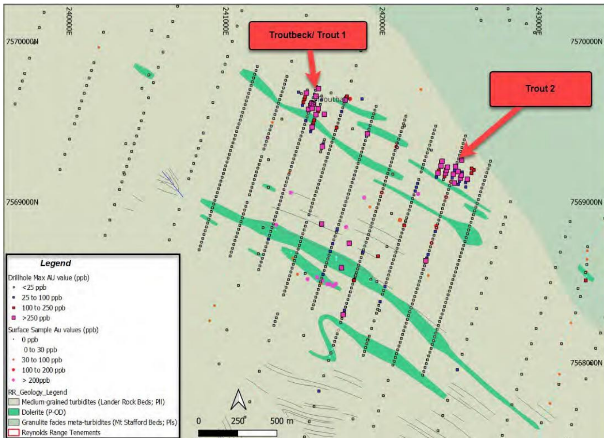
Figure 19. Map of Troutbeck (Trout 1&2) Prospect with drillhole and surface Au values overlying local geology.
