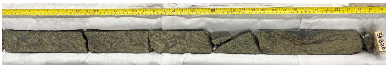
Photo 1. Massive sulphides in drill core from hole ANT0131 at the Antler Copper Deposit in Arizona, USA. This 1.0m interval assayed 18.7% Cu, 5.4% Zn, 1.3% Pb, 85.4 g/t Ag and 1.82 g/t Au (21.0% Cu-Equiv.) from 367.2m down-hole, within a broader 2.5m interval that assayed 10.0% Cu, 4.2% Zn, 1.1% Pb, 55.5g/t Ag and 0.99 g/t Au (2.5m @ 11.8% Cu-Equiv.).
