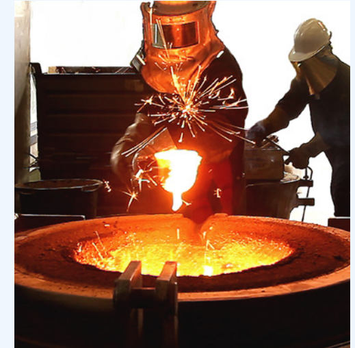
BHP Centre for Sustainable Steelmaking Research conducting a laboratory electric smelting furnace test
