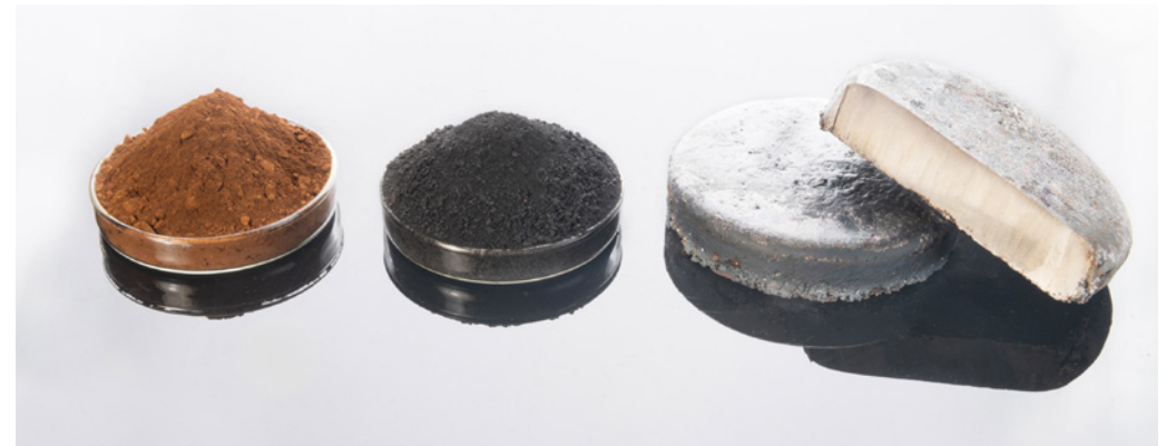
BHP iron ore (left), direct reduced iron produced from BHP iron ore (middle) and iron after electric smelting of BHP direct reduced iron (right)
