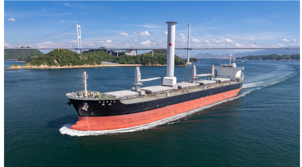
The retrofit installation of a wind rotor on a BHP-chartered vessel, with our partners Pan Pacific Copper and Norsepower
