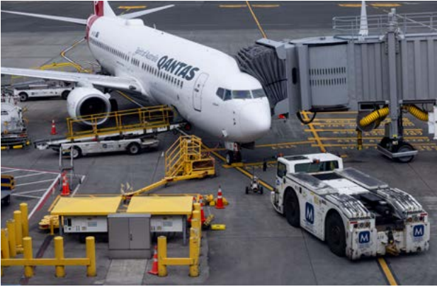
1 Ground power units allow aircraft to connect to New Zealand's low carbon electricity supply instead of burning jet fuel while at the gate.
