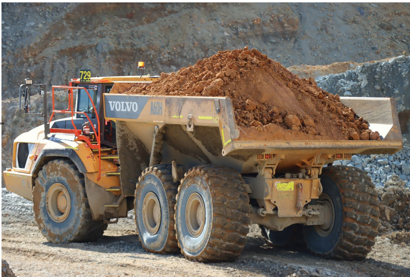
Figure 2. One of the two Volvo A60H 55-tonne dump trucks that have been purchased for trialing at Simberi prior to making the final decision on the choice of truck for Sulphide mining operations.
