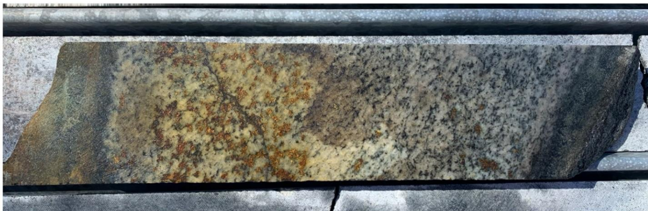
FIGURE 3: GOLD/COPPER INTERSECTION LJPD0032: 0.2M @ 2.26G/T AU AND 2.36% CU HOSTED WITHIN A COARSE GRAINED INTRUSIVE
