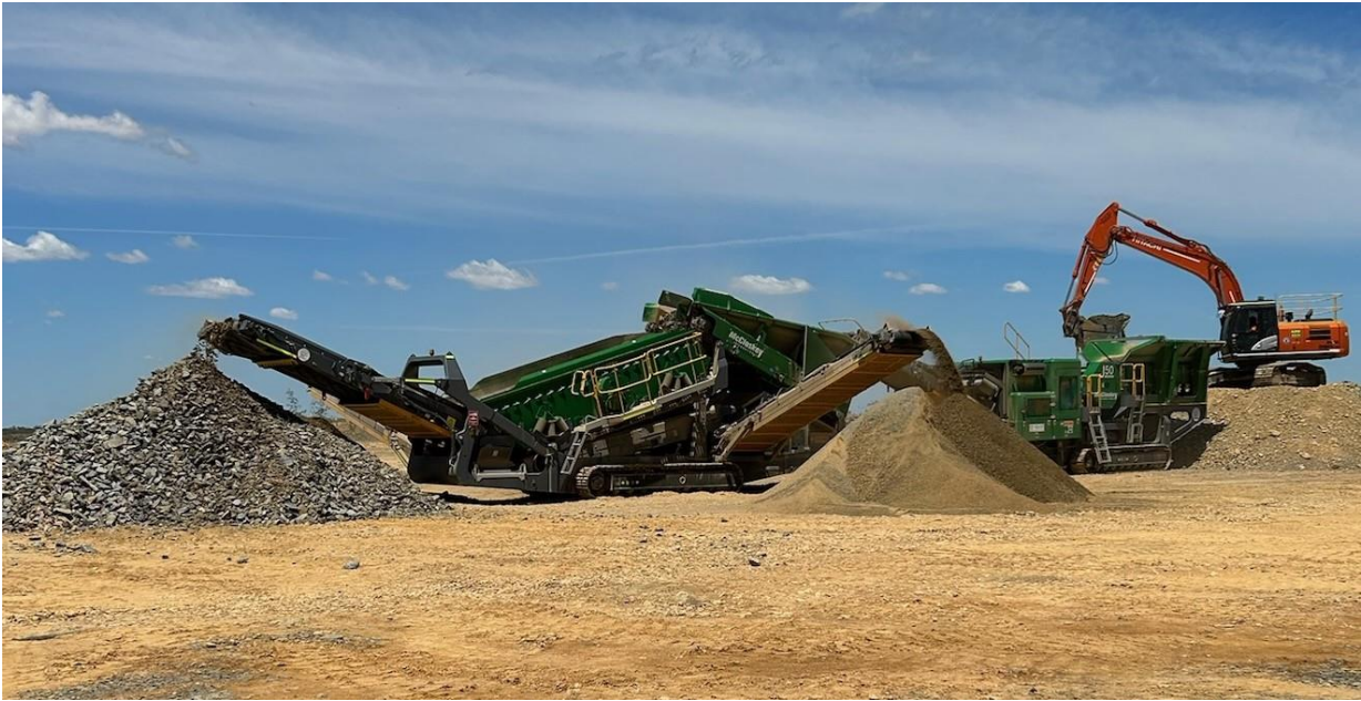
Figure 5: Photo of the McCoskey R230 ‘reclaimer’ mobile screening plant at Mt Boppy.
