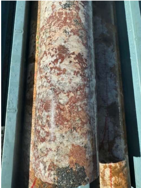
Figure 9: Red rare earth carbonate mineral grains observed in MWDD10101 @ ~70m below surface
