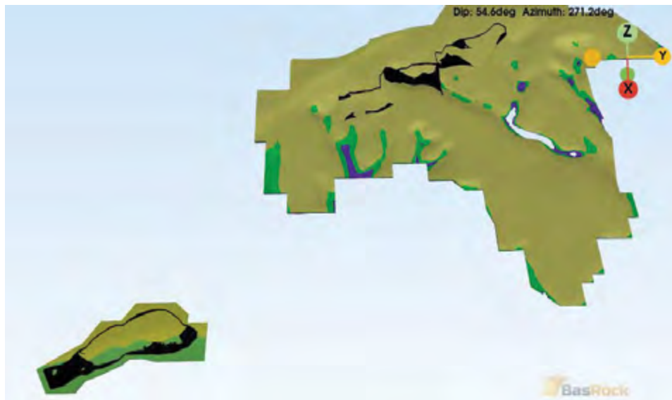
Figure 2.1 Pit outlines and ore solids for Kwale North Dune (top right) and Bumamani (bottom left)
