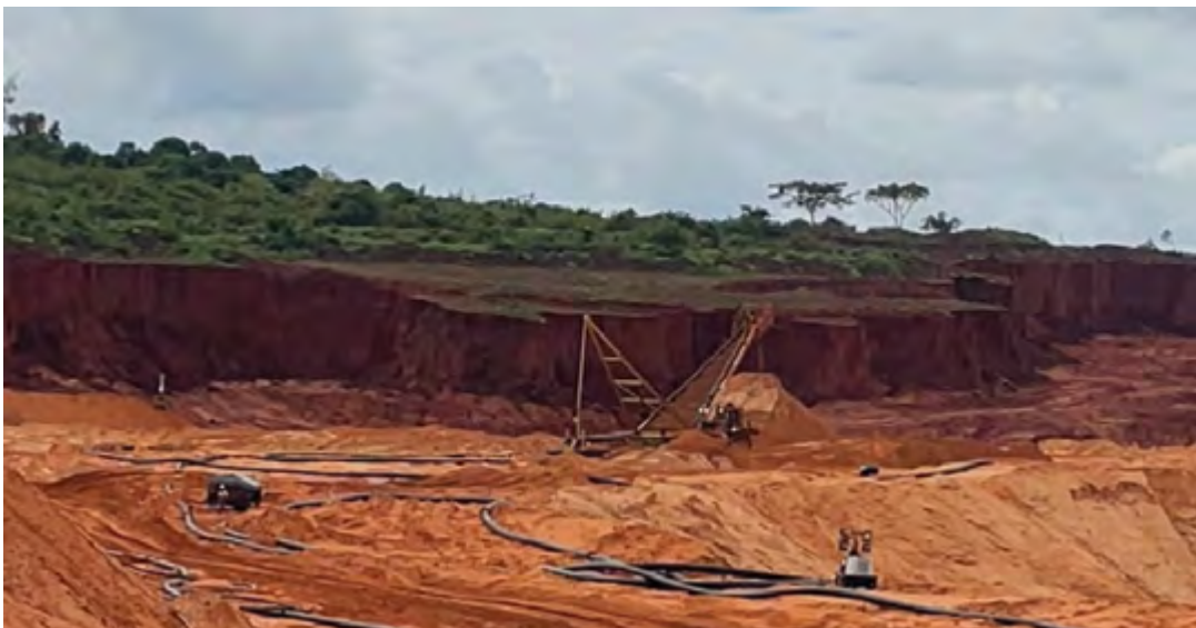
Figure 2.3 Pit edge slope at Kwale showing signs of instability (ravelled material at slope toe, subsiding blocks)
