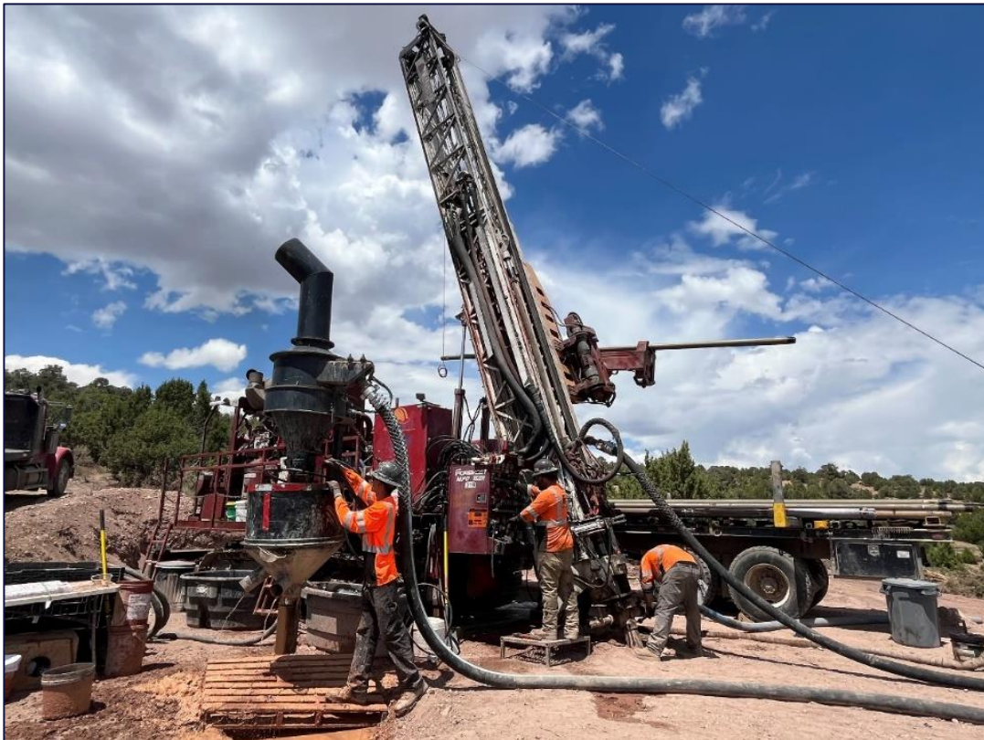
Figure 1 - Alford RC Drill Rig at Maverick Springs
