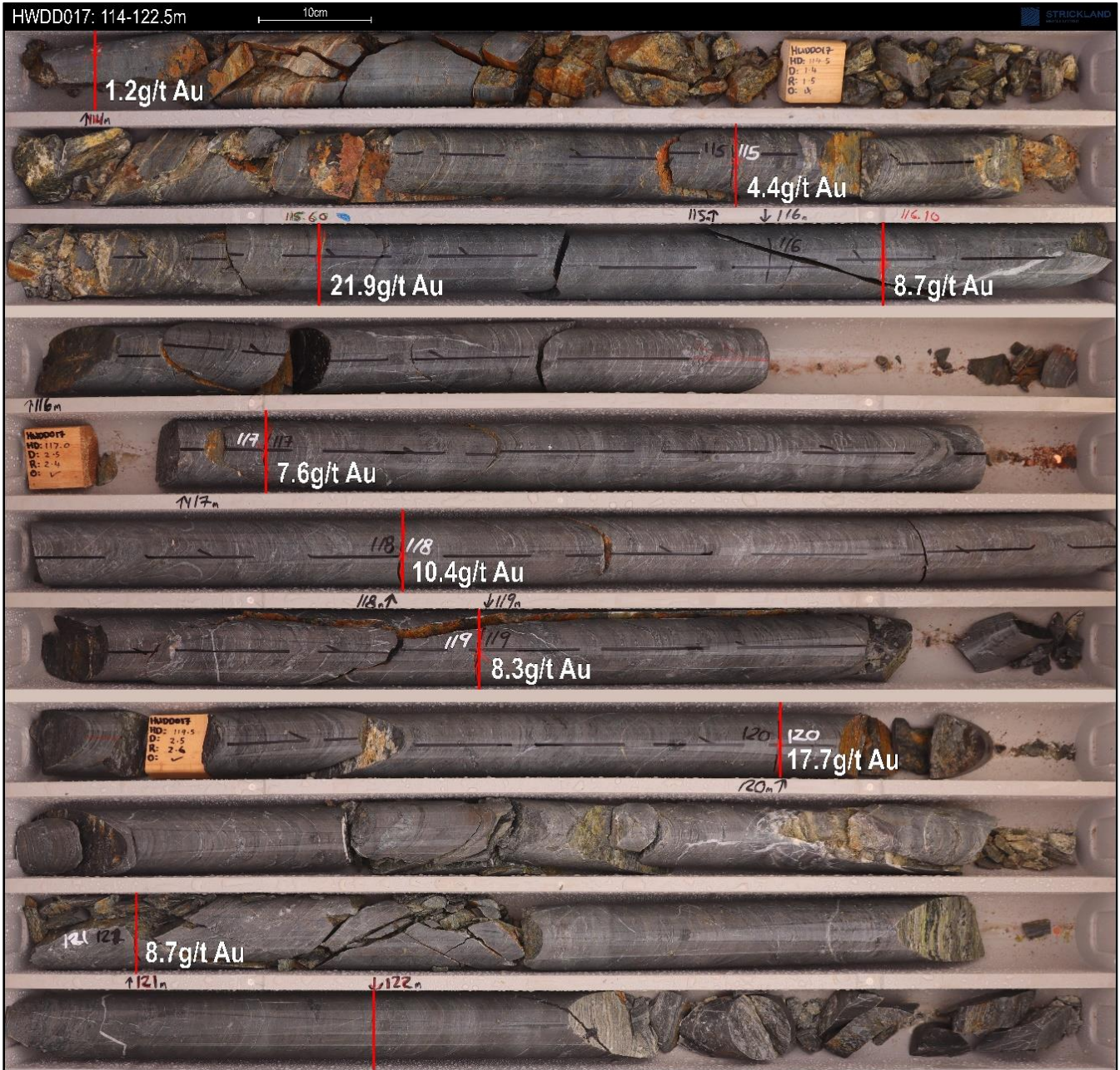
Figure 2. HWDD017 diamond drill core. 114 to 122.5 metres showing the sample intervals (red lines) with the corresponding gold grade in grams per tonne – (lode associated with 14.4 metres @ 6.0g/t Au from 114 metres (including 7 metres @ 10.6g/t Au)
