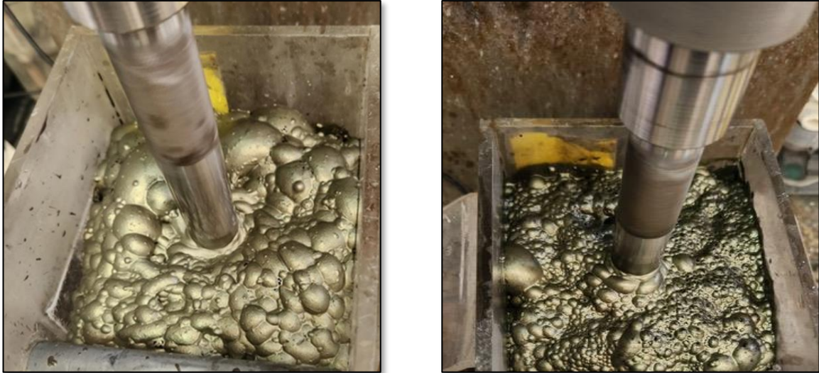
Image 2: Cleaner Flotation Concentration of Chalcopyrite from BBDD0045, Bluebird
