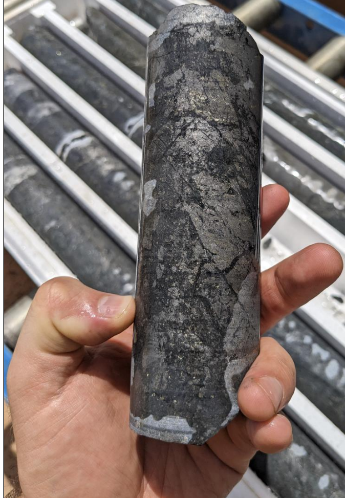
Figure 7: Strong sulphide (arsenopyrite and pyrite) development in mineralised core – HEDD316, 630m (from interval of 35.4m @ 2.8g/t Au)
