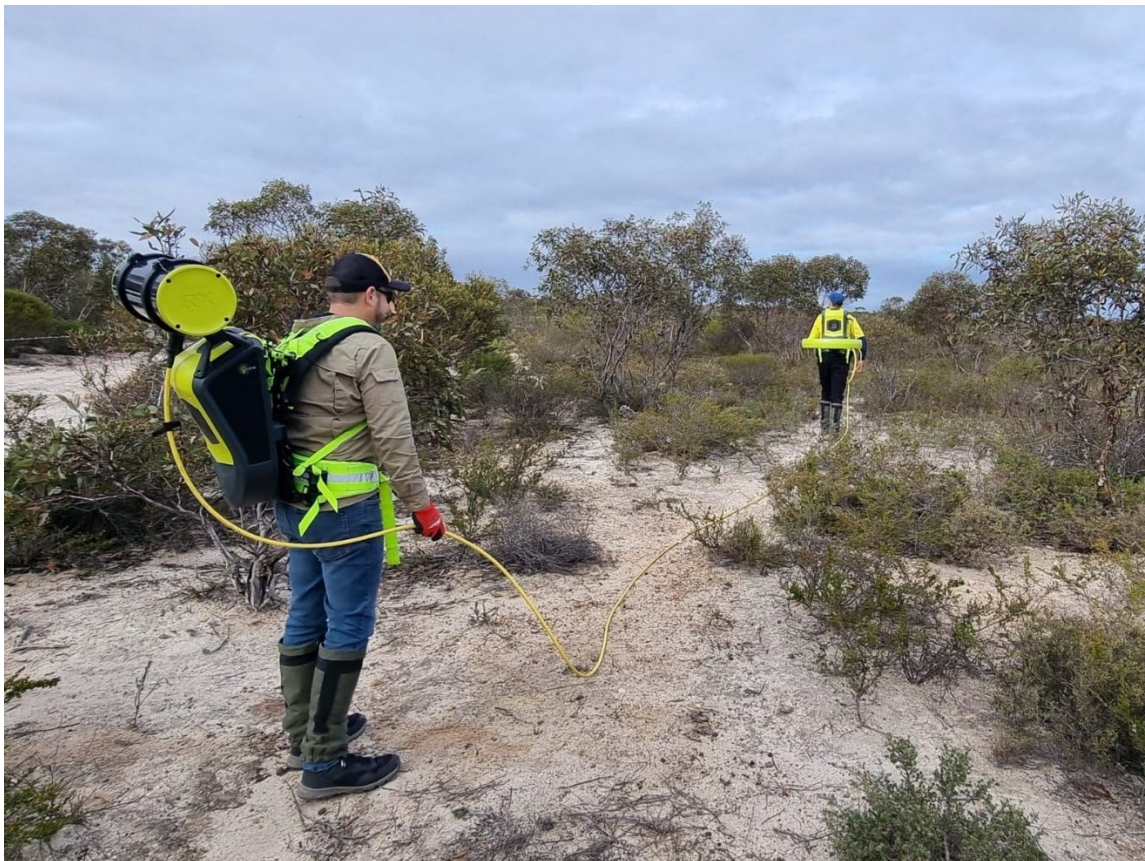
Figure 3: Trial reconnaissance Loupe EM survey being conducted at Quarry North anomaly
