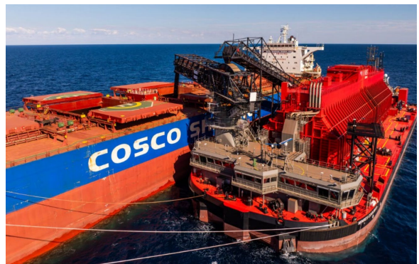
Transhipper discharging ore to minicape vessel
