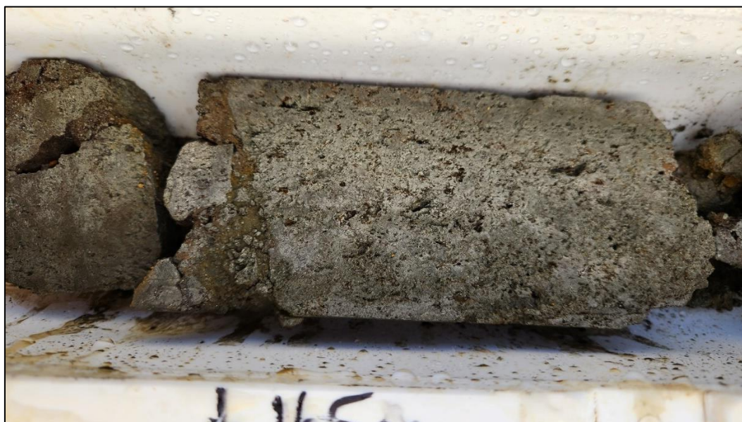
Figure 8. Drillhole MLJDD018 from 164.5m showing Massive pyrite in Breccia
