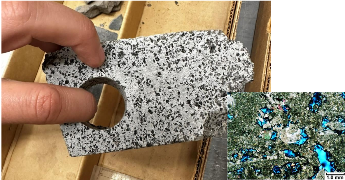
Figure 3: Core from the Lisbon D-616 well (8,619' depth) showing exceptional dolomitic vuggy porosity. Note core plug sample (circular hole). Semi-inset: Thin section at 8,619' showing a 100% dolomite reservoir, with secondary porosity enhanced by hydrothermal dolomitization (pore spaces in blue)
