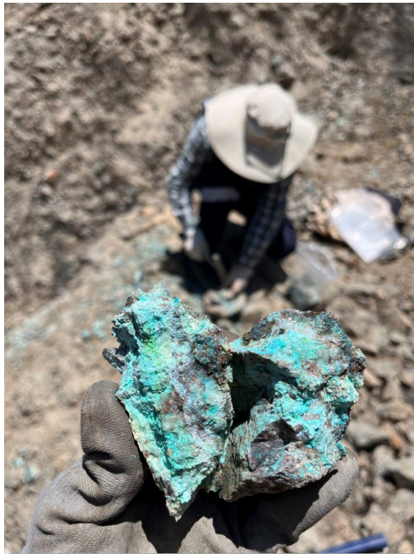
Figure 2: Grab sample 17181 (1.00% Cu) with copper oxides from outcropping historical workings at Cinto Project (see Appendix 1 for details) 2
