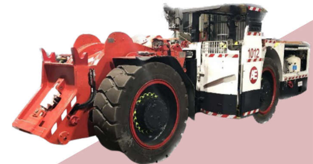
Underground LHD Loader
