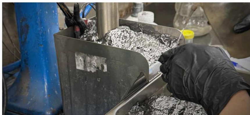
Figure 1. 94% TGC concentrate produced from the Lacroma Deposit
