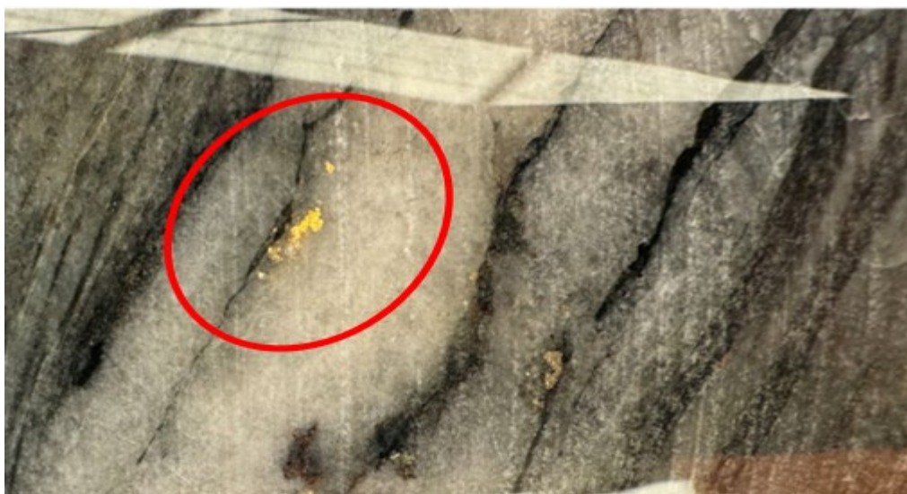
Figure 4: Example for illustrative purposes of coarse gold mineralisation at Gilmour from recent diamond drilling. Photo is approximately 4 cm high.
