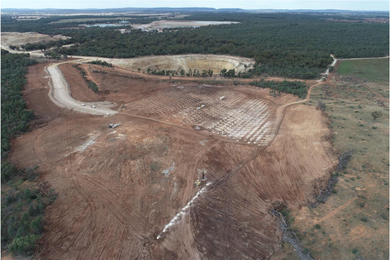
Figure 1: Pearse North – surface cleared, and first pattern drilled out, Pearse South open pit shown in the background. Mining initially commences in Pearse North and a cut back will commence on Pearse South.
