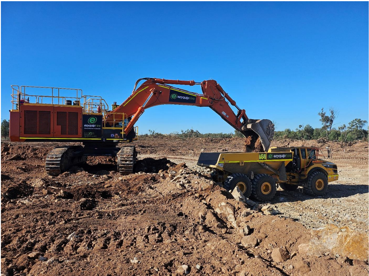
Figure 4: Open pit excavation and haulage.
