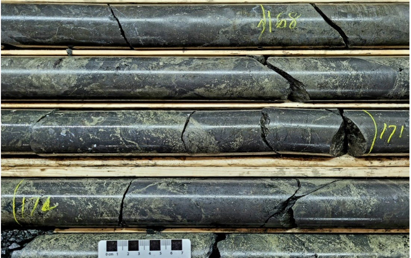
Figure 7: Close-up photo from 7.4 m-long VMS intersection in DDH YH21-22 from 166.6 to 174.00 m- Massive Chalcopyrite, Sphalerite and Pyrite Sulphide Mineralisation
