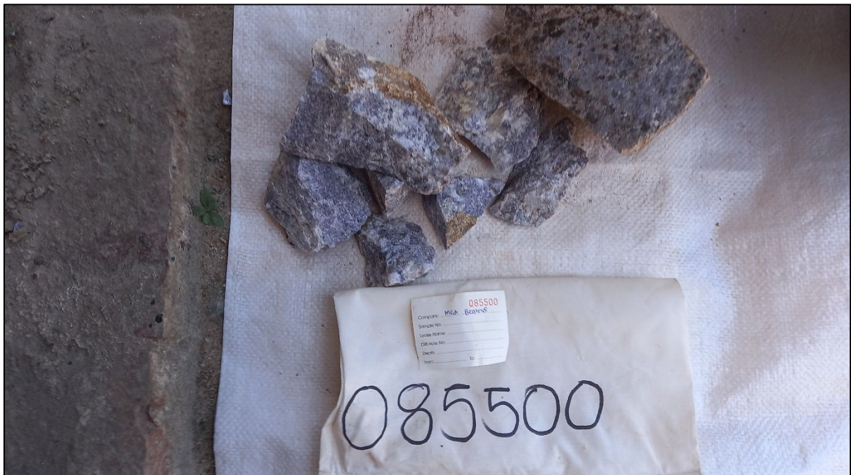
Figure 6: Rock chip sample ID: 85500 From MGA Tenement 0.85% Li 2 O.
