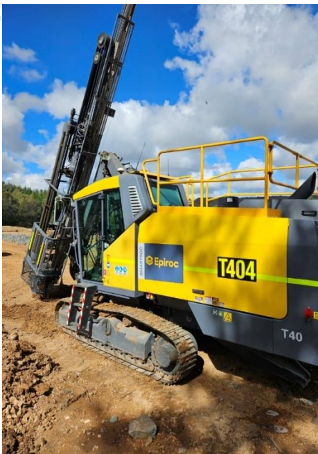
Figure 5: Open pit production drill rig
